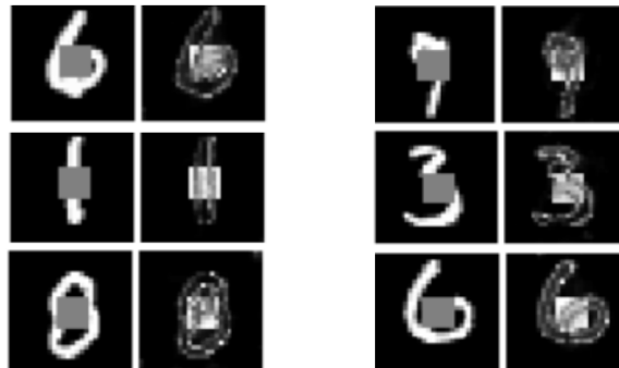
Figure 19: Anomalous images (first column) and it's mean anomaly density map (second column) for six first images of MNIST test set. White indicates big difference and black indicates no difference.
