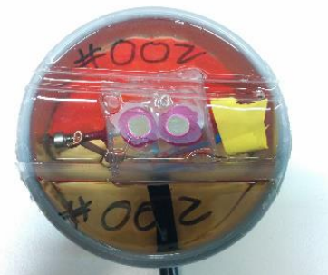
Figure 5 Potentiostat device. Three electrode cell with waterproof enclosure
