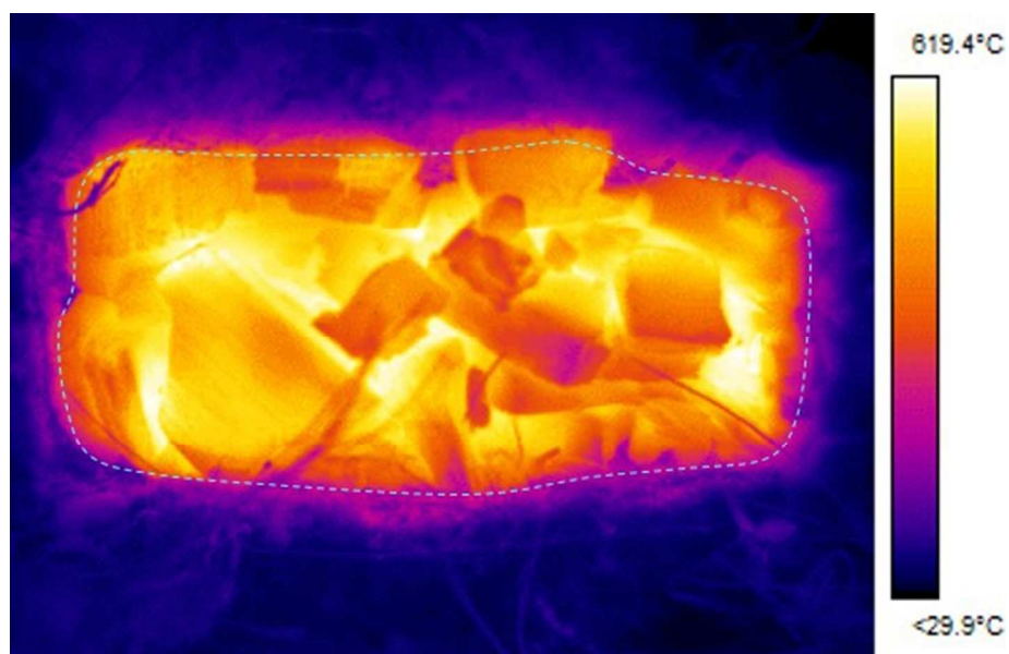
Fig. 5. b) Temperature distribution of burning charcoal at the beginning of test (randomly selected W2_B4). Blue dashed line delimits the 30 cm x 10 cm surface area occupied by charcoal. Mean temperature of the delimited area is 434°C (st.dv is 95.3°C)
