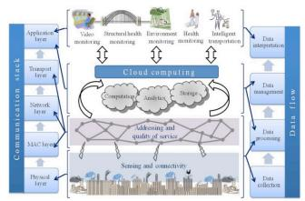
Fig. 3. Example of cloud based information framework for smart cities<sup>1</sup>.
