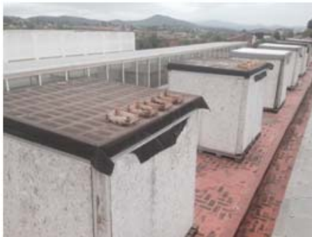
Figure 3. Overview of selected modules of the various boxes of crushed glass, placed on respective decks no. 1, 2 and 3
