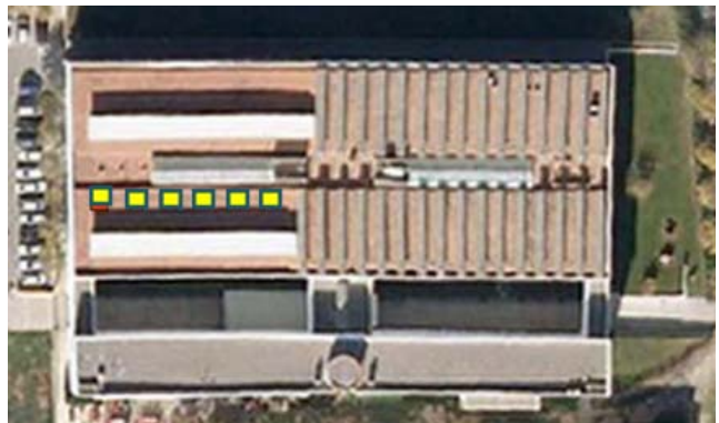
Figure 02. Aerial view of the position of measurement cubes on the deck of the Vallès School of Architecture
