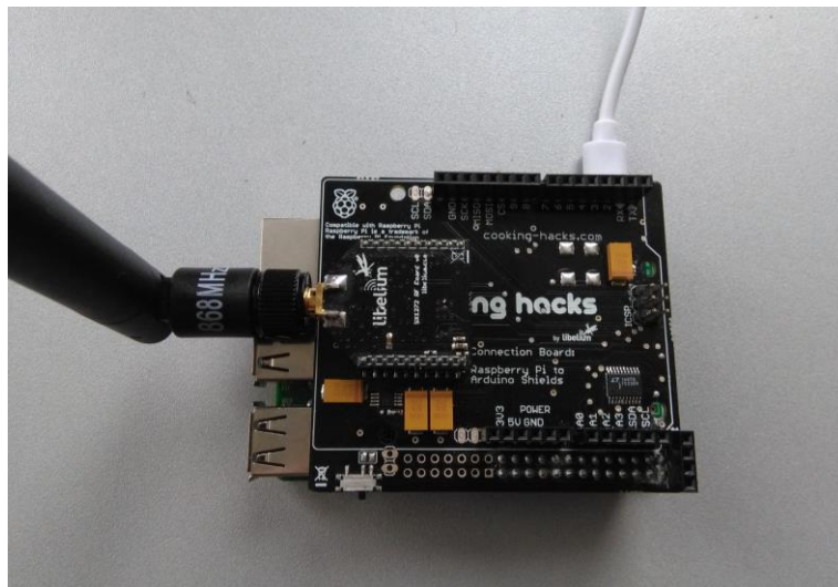
Figure 22. Gateway completely assembled
