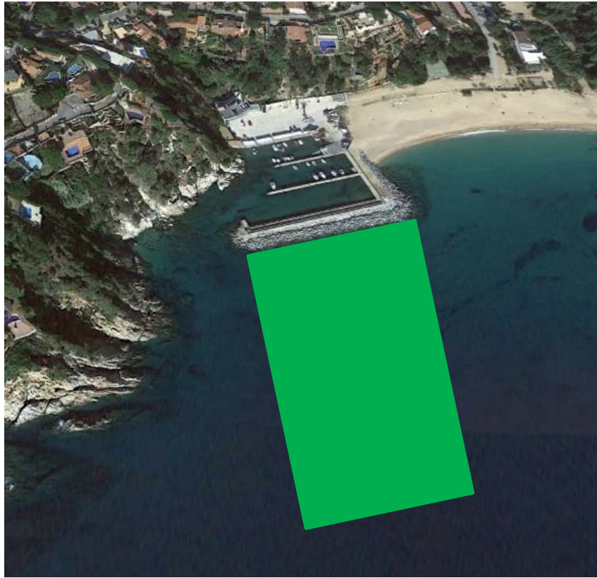
Figure 3. Lay-out of the proposed seagrass meadow in front of Cala Canyelles harbour, illustrating a “green” intervention to reduce overtopping under future climates.
