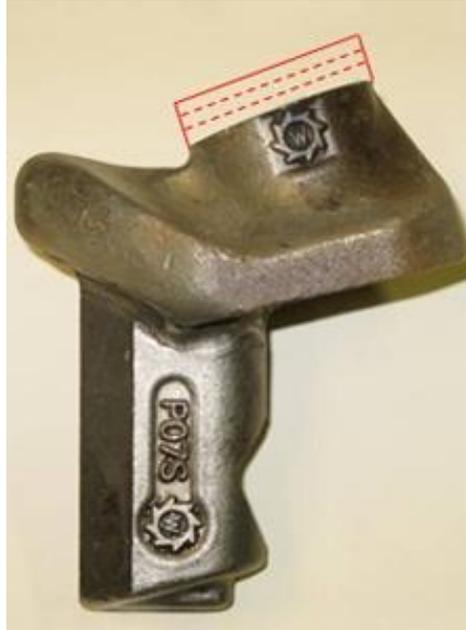
Gambar 5 *Parallel wear to the contact surface*
