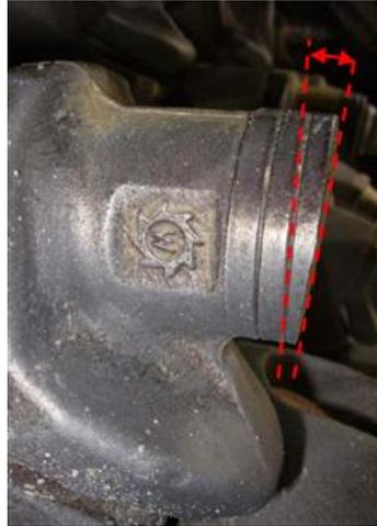
Gambar 6 *Wedge-shaped wear inwards toward the contact surface*
