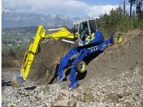
Gambar 10 Spider Excavator Kaiser S2 4x4 Cross
