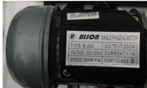
Gambar 1. Data nameplate dibodi motor.
