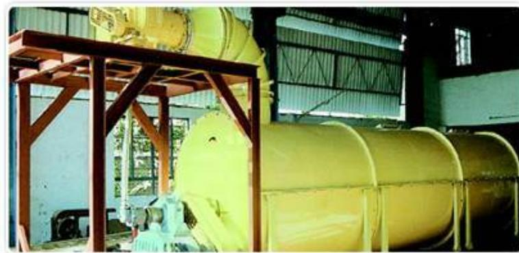
**Gambar 5.** *Conduction dryer* (Sari : 2012)
