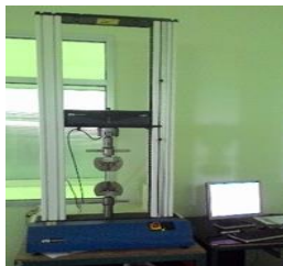
Gambar 5. Universal Testing Machine (Instron 3367)
