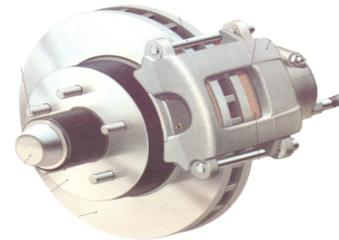
**Gambar 6.** Rem Cakram (<http://www.motorera.com/dictionary/DI.html>)
