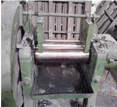
**Gambar 2 .** Mesin *Two Roll Mill*
