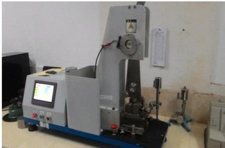
**Gambar 8.** Alat Uji Izod Impact
