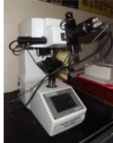
**Gambar 10.** *Micro Vickers Hardness Machine*
