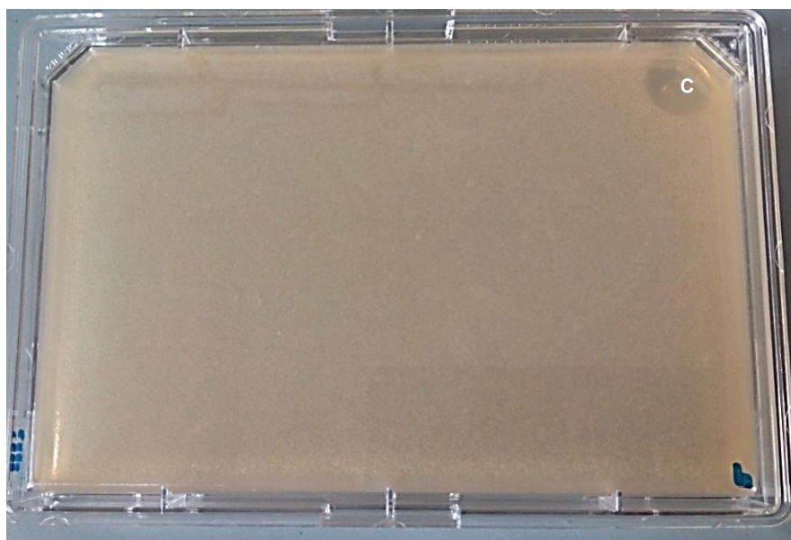
Fig. 18– Modified Kirby-Bauer assay with small scale extracts of Planctomycetes (from M600 cultures) tested against M. luteus after 24h incubation at 37° C. The control was 10 \mu L of 1 \mu g/mL ampicillin (C). No inhibition halos were observed for any extract.
