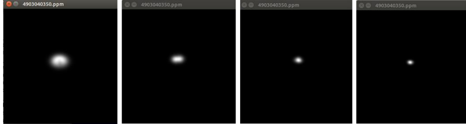
Fig. 4. Evolution of an iBeacon (id = 4903040350) Grid Map with 0.25meters/pixel resolution
