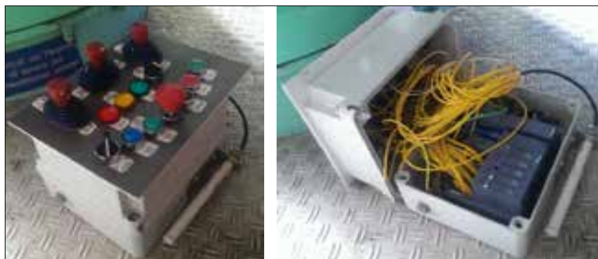
Figure 5. Operating console for the remote control of the mobile hydraulic platform
