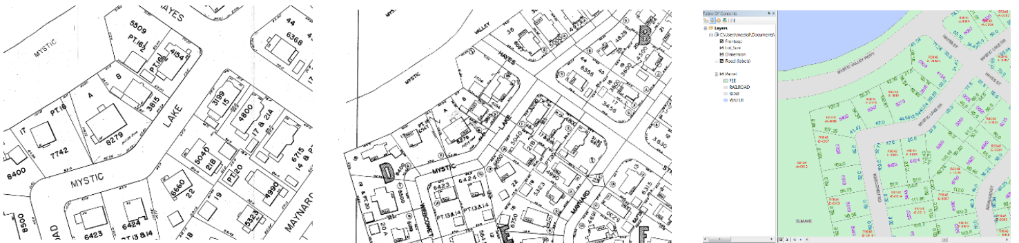
Figure 6. The engineer, assessor, and GIS map comparing the dimensions of the parcels to one another. The goal of this comparison was to make the GIS maps as up to date and accurate as possible.
