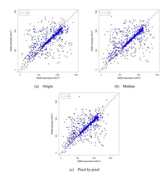
Figure 28 The scatter plots of ground measurements versus DSSR estimates for three different cloud structures. Parallax effect was not corrected in (a). Parallax effect was corrected by a median value of the horizontal displacements of the scene in (b). Parallax effect was corrected pixel by pixel in (c).
