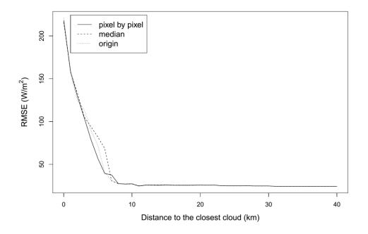
Figure 36 The plot of DCC versus RMSE for the three cases to examine parallax effect. The y axis value is the bias of scenes that DCC is greater than the x axis value.
