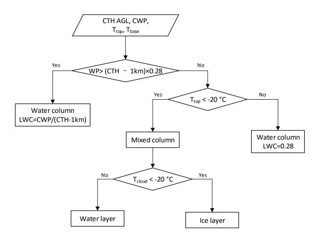
Figure 15 The flowchart to determine the types of cloud
