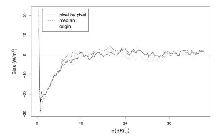
Figure 30 The plot of DSSR variability versus bias for the three cases to examine parallax effect. The y axis value is the bias of scenes that DSSR variability is less than the x axis value.
