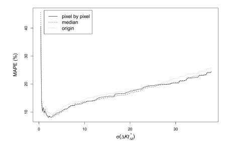
Figure 32 The plot of DSSR variability versus MAPE for the three cases to examine parallax effect. The y axis value is the MAPE of scenes that DSSR variability is less than the x axis value.
