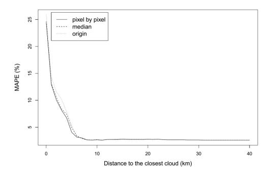
Figure 37 The plot of DCC versus MAPE for the three cases to examine parallax effect. The y axis value is the bias of scenes that DCC is greater than the x axis value.
