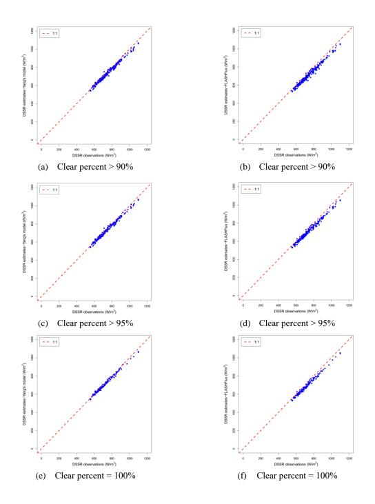
Figure 27 The comparisons between DSSR derived from Yang's model and FLASHFlux with three clear percent thresholds. (a), (c), and (e) are scatter plots of ground measurements versus DSSR estimates using Yang's model; (b), (d), and (f) are scatter plots of ground measurements versus DSSR estimates of FLASHFlux
