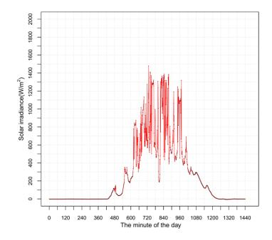
Figure 6 Minutely (GMT+8) solar irradiance scatterplot on July 13th, 2012
