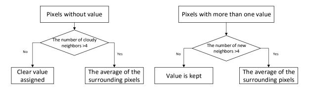
Figure 12 Flow chart of gap correction
