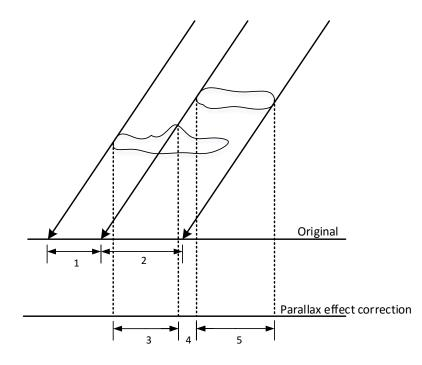
Figure 10 Possible gap results from parallax correction. No.1 and No.2 areas are the projection of the cloud in from a satellite viewing angle. No.3 and No.5 areas are the vertical projection of cloud after parallax correction. No.4 area is the gap.
