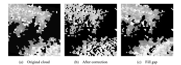
Figure 11 Gaps appearing on the image due to parallax correction
