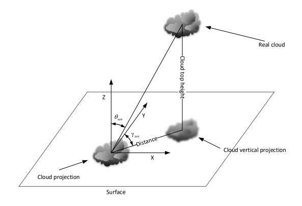
Figure 9 Principle of parallax correction. The horizontal displacement of the apparent position is a function of the cloud base height and satellite zenith and azimuth angle. A correction becomes necessary if the distance between the apparent and the true location exceeds the spatial resolution (Wyser et al. 2002).
