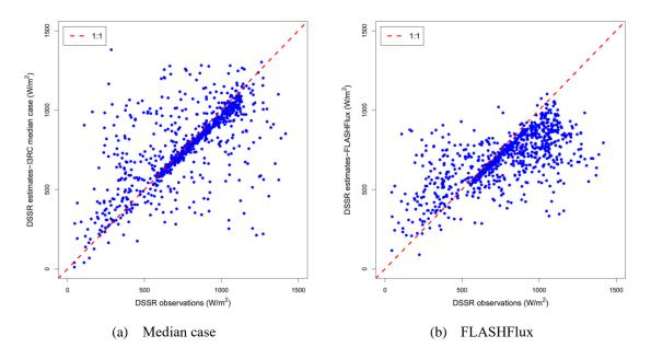
Figure 39 Scatter plots of ground measurements versus DSSR estimates of median case and FLASHFlux for all-sky conditions
