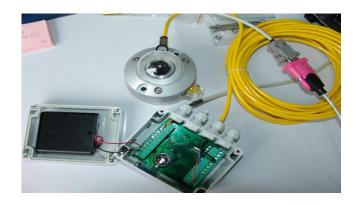
Figure 4 The connection of CMP-6
