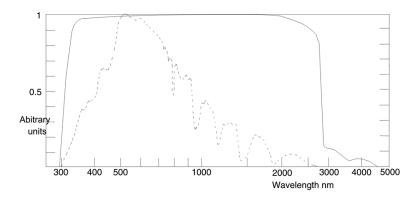
Figure 5 Solar irradiance spectrum at the Earth's surface and pyranometer response (CMP-6 user manual)
