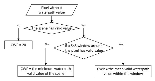
Figure 17 The flow chart to assign CWP value to the pixel without CWP value
