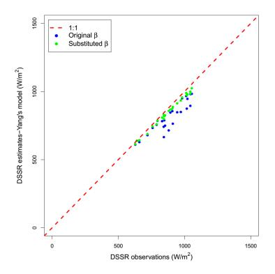
Figure 25 Scatter plots of ground measurements versus DSSR estimates using Yang's model when clear percent is greater than 90% and original  $\beta$  are greater than 0.0256
