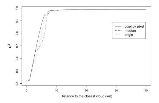
Figure 38 The plot of DCC versus  $R^2$  for the three cases to examine parallax effect. The y axis value is the bias of scenes that DCC is greater than the x axis value.
