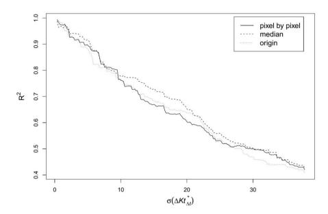
Figure 33 The plot of DSSR variability versus  $R^2$  for the three cases to examine parallax effect. The y axis value is the  $R^2$  of scenes that DSSR variability is less than the x axis value.
