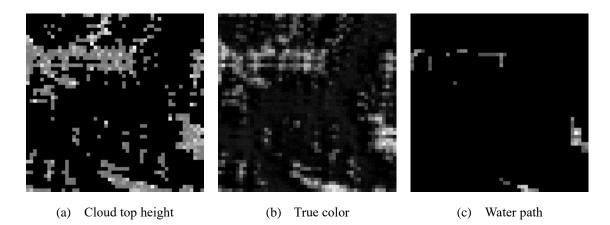
Figure 16 The data missing problem of MOD06. The three images were derived from MODIS image at 6:45 AM GMT the 271<sup>st</sup> day in 2012. The coordinates of the center pixel of the image is (1180, 32). The gray or white color of the pixel in the three figures means the pixel has value.
