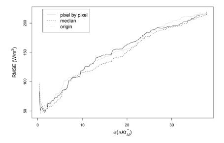
Figure 31 The plot of DSSR variability versus RMSE for the three cases to examine parallax effect. The y axis value is the RMSE of scenes that DSSR variability is less than the x axis value.
