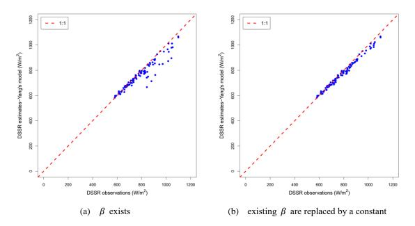
Figure 24 Scatter plots of ground measurements versus DSSR estimates using Yang's model when clear percent is greater than 90%
