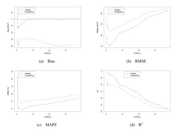
Figure 40 The plot of DSSR variability versus four statistical indices for DSSR estimates of median case and FLASHFlux. The y axis value is the statistical indices of scenes that DSSR variability is less than the x axis value.
