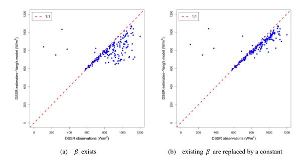
Figure 23 Scatter plots of ground measurements versus DSSR estimates using Yang's model
