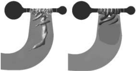
Figure 9: Vortex flow structure in the draft tube of the aerodynamic turbine (DES, RSM)
