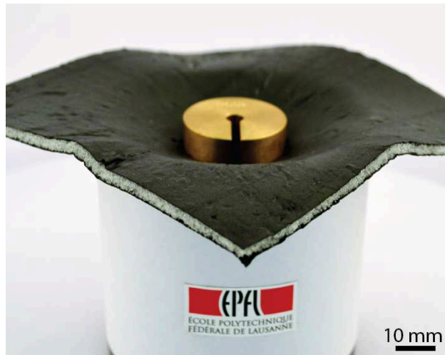
Fig. 1. The soft monolithic silicone-based capacitive sensor skin deforming into a mug. The sensor skin measures 120 \times 120 \times 4 mm 3 with 70 pF of overall capacitance.
