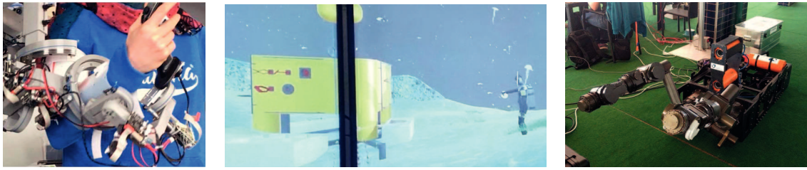
Figure 6.2: Teleoperation setup to control ROV: ( left ) exoskeleton and the virtual reality headset worn by the teleoperator, ( middle ) third person view of the teleoperator in the virtual reality environment, ( right ) ROV with manipulator controlled by the teleoperator.
