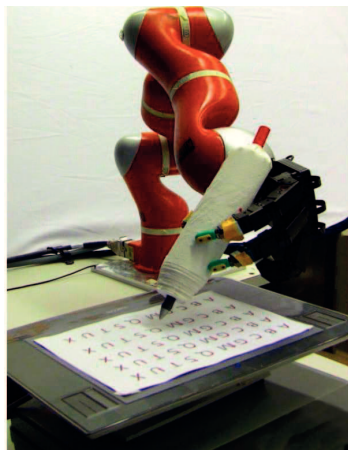
Figure 2.14: Letter writing setup with the KUKA robot.
