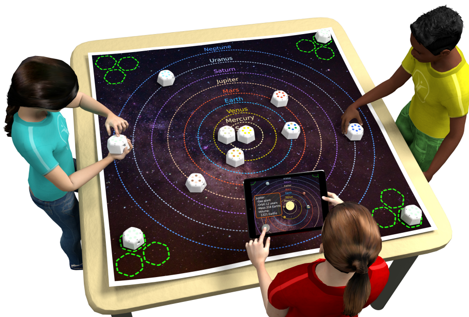
(a) Solar System : Robots simulate planets orbiting the sun. Learners can tangibly move the planets to alter their orbits or even attempt to remove the sun to see what happens when the major source of gravity disappears.
