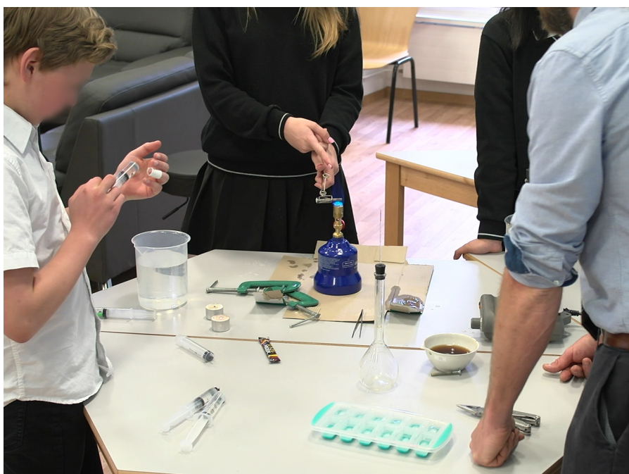
(b) Practical activity. Same team of learners experimenting with states of real-world matter using common laboratory equipment. On the left, learner attempting to compress the liquid in a syringe, which is not possible. In the middle, learner heating a bolt on the Bunsen burner, to later tightly clamp it and rapidly cool it (via soaking it in water) in order to observe contraction through changing temperature which will release it from the clamp.
