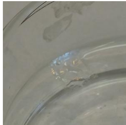
Figure 9: Result of the etching with PMMA on the top. We can see that the structure is not flat, there is a deformation.
