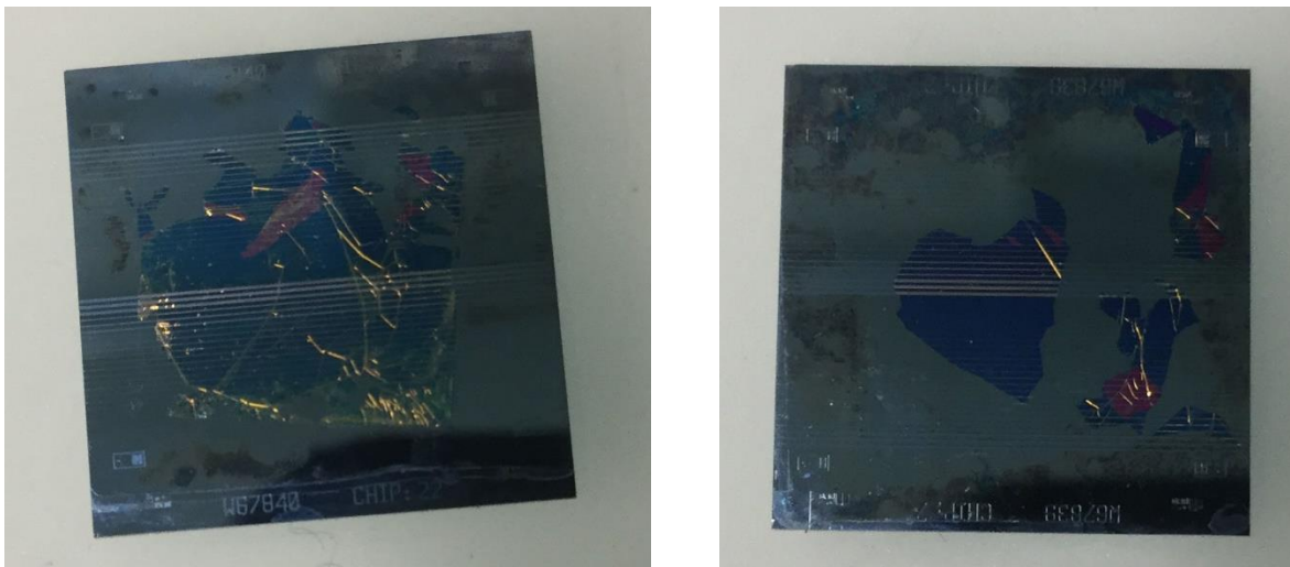
Figure 24: Pictures of the backside transference result. At left side, we have a chip with less folds than the second try. At the right side, we have a test without folds and bigger flat parts (the microscope images demonstrated that this test was not so efficient).
