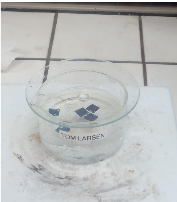
Figure 7: Chips prepared in KOH solution to be etched. Hot plate temperature 80°C.
