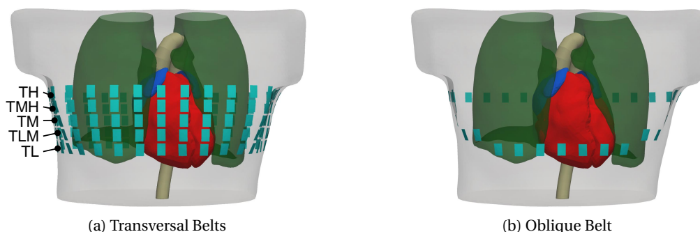
Figure 4.1 – 4D bioimpedance model of the human thorax with (a) transversal and (b) oblique electrode belt placements (see text Section 4.2.2). The EIT electrodes are shown in light blue. The static thorax model contains the following dynamic structures: heart with atria (dark blue) and ventricles (red), aorta (gray) and both lungs (green). Please note that for the sake of clarity only 32 (instead of 64) electrodes are shown per belt.
