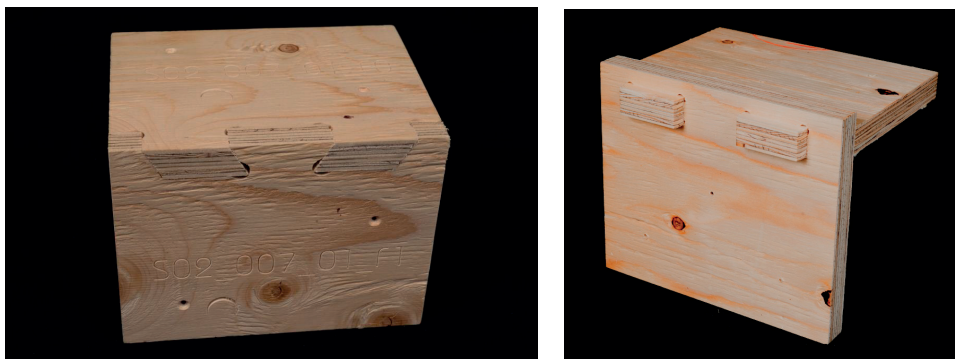
Figure 4.21 – MTSJ: open slot (left), closed slot (right).
