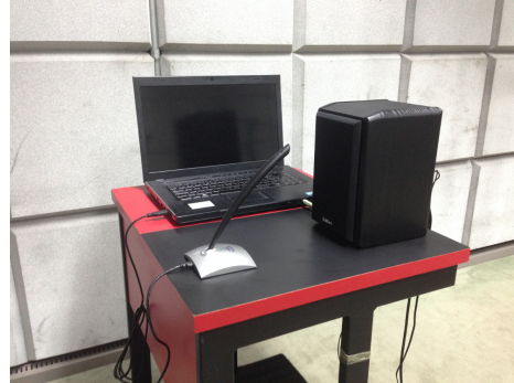
Figure 2. Example of BioCPqD-PA database recording setup. All attacks were recorded in an acoustically isolated room.
