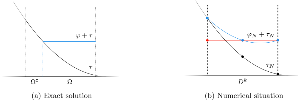
Figure 4: Comparison of the exact and numerical “lake at rest” solutions. The polynomial approximation cannot have a vanishing slope unless unphysical, negative water heights were to be allowed.
