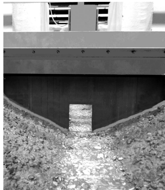
Fig. 3. Picture of the channel with constriction composed of multiple PVC elements (view from upstream to downstream)
