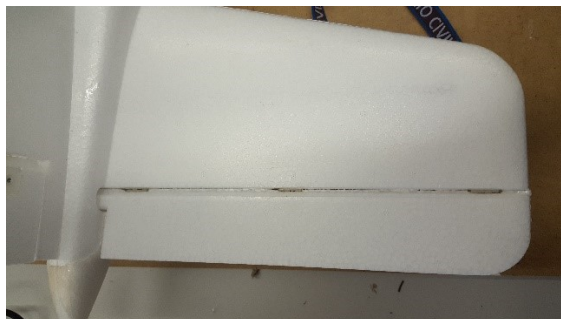
Figure 5: Elevator attached with (white) plastic hinges, which are glued into the frame and edge of the elevator surface.
