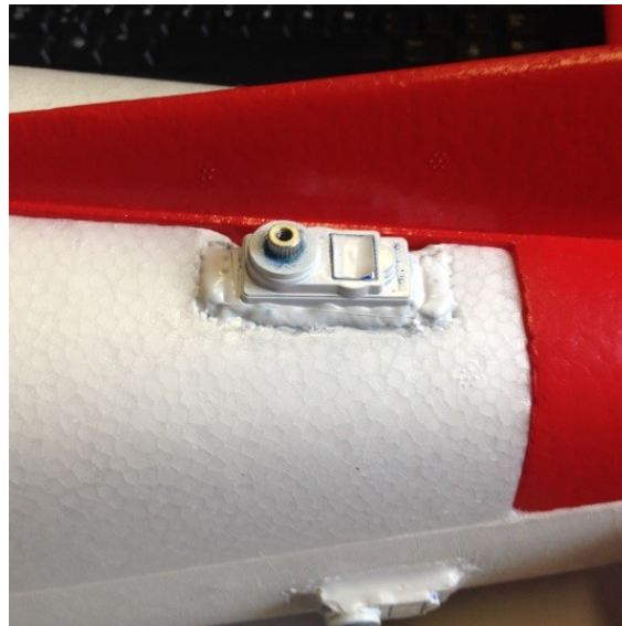
Figure 3: Waterproof servomotors installed with mastic.
