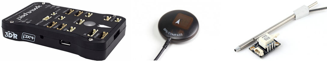
Figure 6: Autopiloting hardware: Pixhawk autopilot, GPS receiver, Pitot tube.
