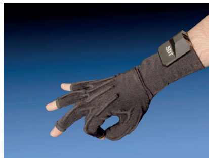
Figure 1.3 – Example of a commercially available wearable motion sensing for the hand: the Data Glove Ultra from 5DT. Picture copyright 5DT.
