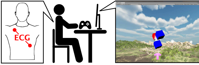
Fig. 2. Setup of the experiment. The subject seats in front of a screen and interacts with the simulator through a gamepad. The electrodes placement on the chest for ECG monitoring is depicted on the left. On the right, a screenshot of the F3M task, namely, flying and mapping 3 objects is shown. The arrow on the image indicates the direction of the next waypoint (white cloud), and the cubes are the objects to be detected by pressing a button of the controller.
