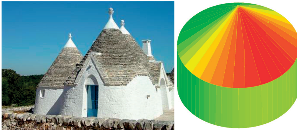
Figure 7.5 Trullo (left). Source: Pintarest. Hourly solar radiation (13:00) during a summer day (right)
