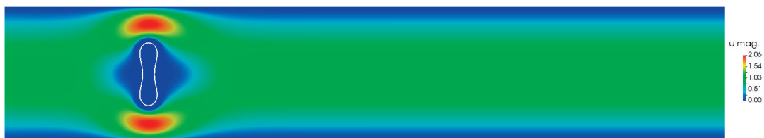
Figure 7.19 – Flow past NURBS obstacle at Re = 20 . Velocity at time t = 20 .
