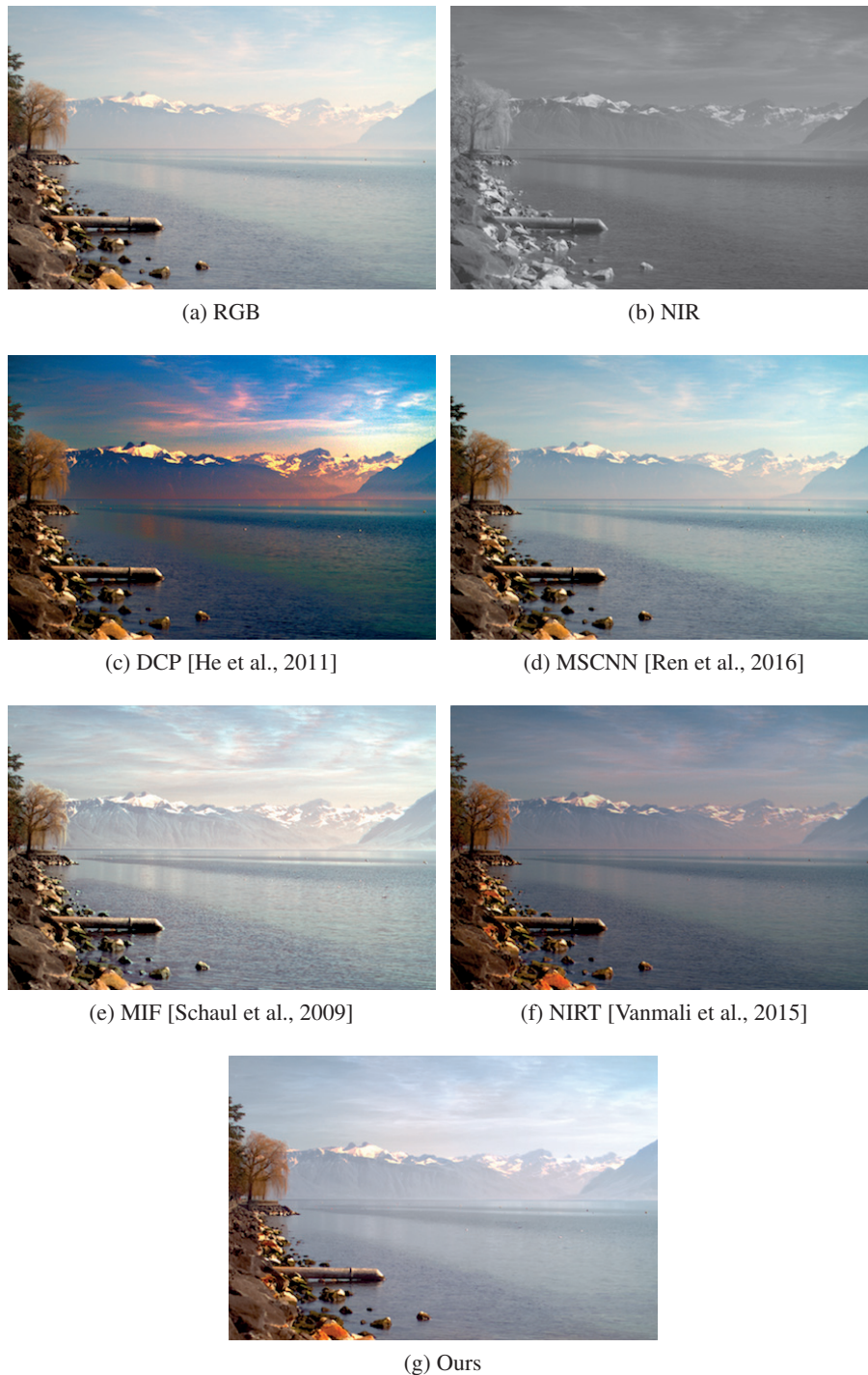
Figure 5.9 – Qualitative comparison with the state-of-the-art in single and visible-NIR haze removal. DCP [He et al., 2011] and MSCNN [Ren et al., 2016] are based on a single image, while MIF [Schaul et al., 2009] and NIRT [Vanmali et al., 2015] use visible-NIR image pairs. Our algorithm is able to faithfully reproduce colors while adding sufficient detail from the NIR image to the output.
