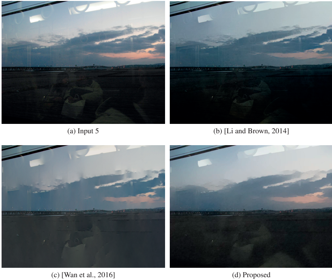
Figure 4.14 – Comparison of reflection removal methods on real-world images taken from the Internet. As in the case of artificial images, the method of [Li and Brown, 2014] suffers from poor color reproduction, while the method of [Wan et al., 2016] over-smooths the image. Our method gives superior color reproduction and reflection suppression results compared to both the state-of-the-art techniques. Best viewed on screen.
