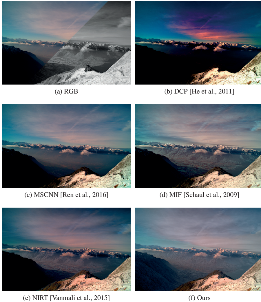
Figure 5.18 – Failure case of the state-of-the-art in single and visible-NIR haze removal. None of the algorithms is able to sufficiently remove the haze component from these challenging images.
