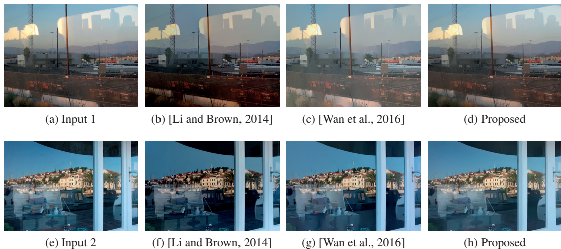
Figure 4.15 – Failure cases in reflection removal. In this figure, we show the cases where our technique fails to suppress reflections satisfactorily. We pose our results next to the results from the state-of-the-art [Li and Brown, 2014; Wan et al., 2016] to show that they are equally unsuccessful in removing reflections. This is due to the fact that the reflection components are too strong to be distinguished from the main transmission layer. Best viewed on screen.
