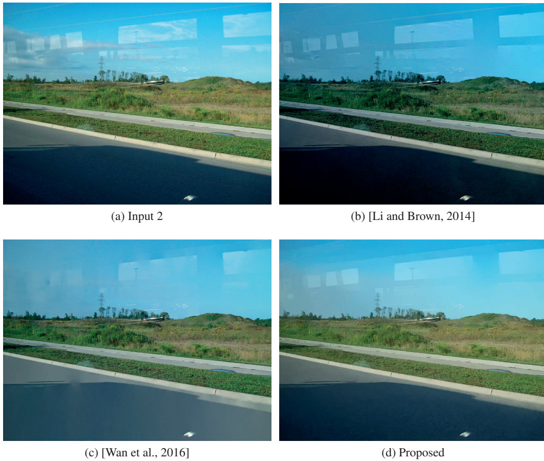
Figure 4.11 – Comparison of reflection removal methods on real-world images taken from the Internet. As in the case of artificial images, the method of [Li and Brown, 2014] suffers from poor color reproduction, while the method of [Wan et al., 2016] over-smooths the image. Our method gives superior color reproduction and reflection suppression results compared to both the state-of-the-art techniques. Best viewed on screen.
