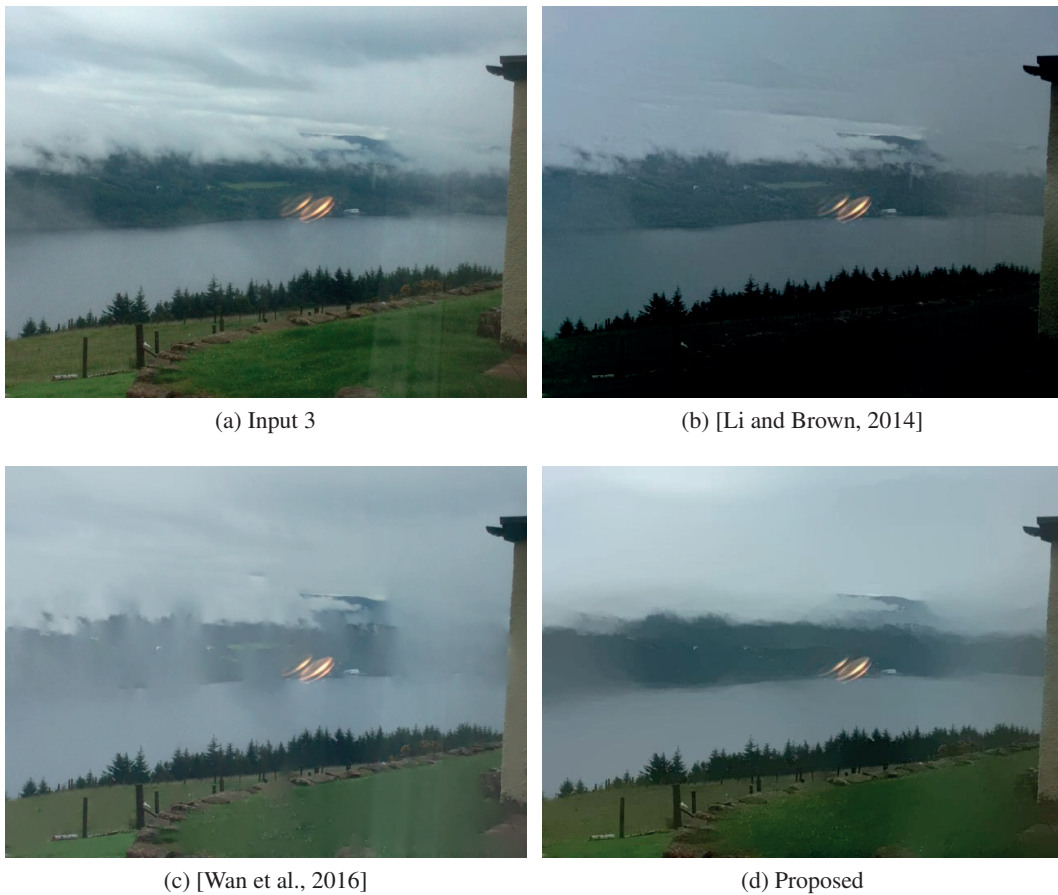
Figure 4.12 – Comparison of reflection removal methods on real-world images taken from the Internet. As in the case of artificial images, the method of [Li and Brown, 2014] suffers from poor color reproduction, while the method of [Wan et al., 2016] over-smooths the image. Our method gives superior color reproduction and reflection suppression results compared to both the state-of-the-art techniques. Best viewed on screen.
