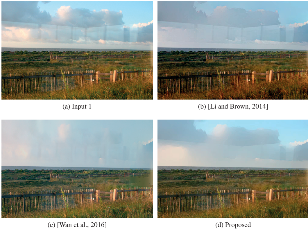
Figure 4.10 – Comparison of reflection removal methods on real-world images taken from the Internet. As in the case of artificial images, the method of [Li and Brown, 2014] suffers from poor color reproduction, while the method of [Wan et al., 2016] over-smooths the image. Our method gives superior color reproduction and reflection suppression results compared to both the state-of-the-art techniques. Best viewed on screen.
