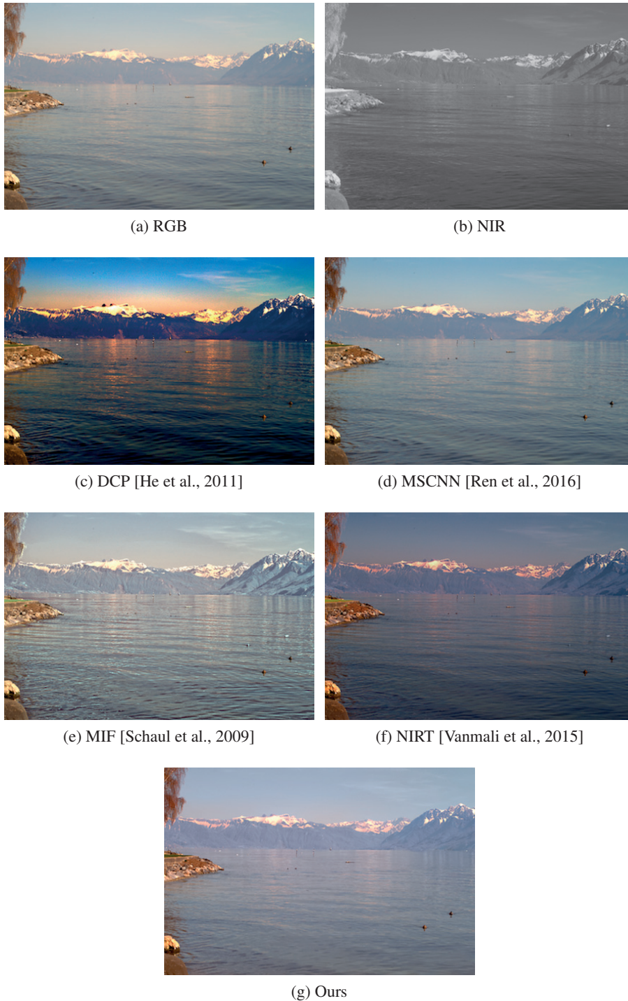
Figure 5.8 – Qualitative comparison with the state-of-the-art in single and visible-NIR haze removal. DCP [He et al., 2011] and MSCNN [Ren et al., 2016] are based on a single image, while MIF [Schaal et al., 2009] and NIRT [Vanmali et al., 2015] use visible-NIR image pairs. Our algorithm is able to faithfully reproduce colors while adding sufficient detail from the NIR image to the output.
