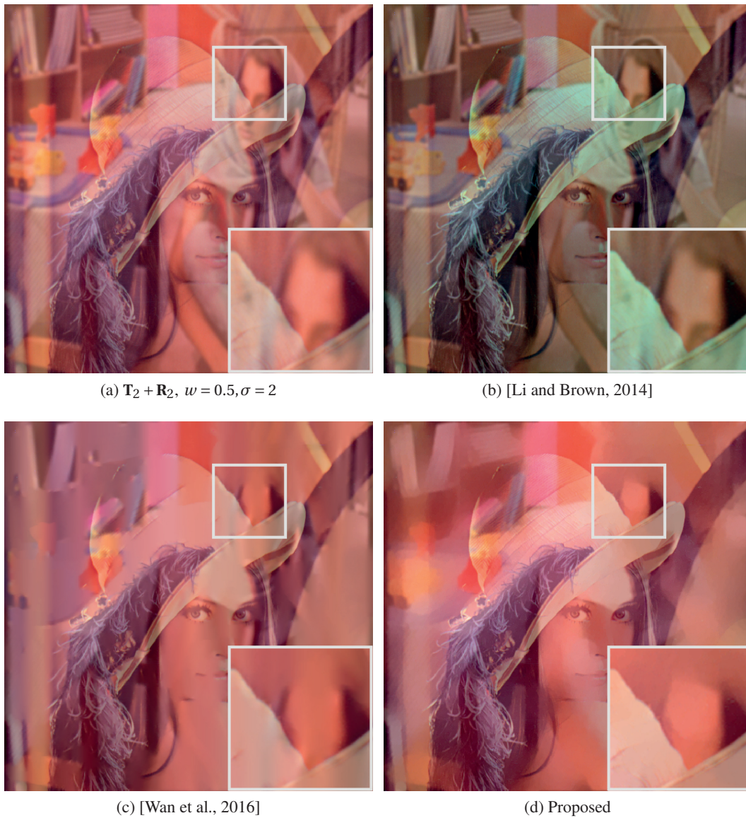
Figure 4.9 – Comparison of reflection removal methods on synthetic images with blending weight w = 0.5 . Compared to [Li and Brown, 2014] and [Wan et al., 2016] our method gives superior color reproduction and reflection suppression results. Best viewed on screen.
