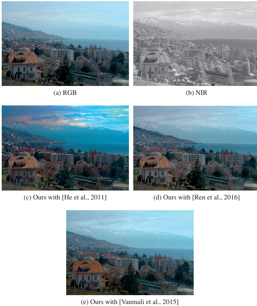
Figure 5.6 – Qualitative comparison of transmission estimation algorithms using our proposed scene radiance estimation. The method of [Vanmali et al., 2015] is in general more accurate with faithful color reproduction. The methods of [He et al., 2011; Ren et al., 2016] result in unrealistic over-saturated colors, particularly on the sky regions of the image.
