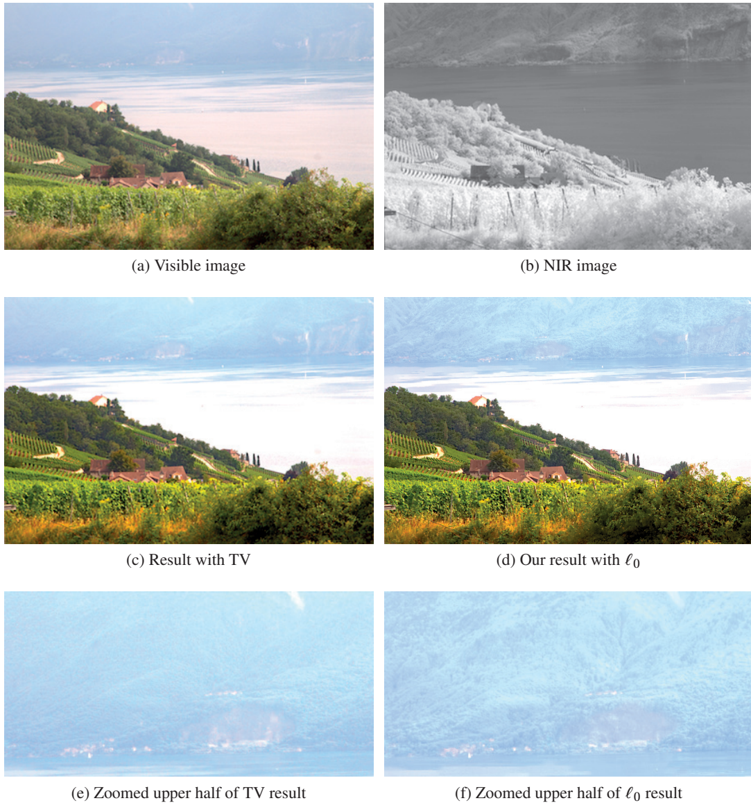
Figure 5.2 – Haze removal results with TV regularization (Fig. 5.2c) and with our \ell_0 regularization term (Fig. 5.2d). Our \ell_0 approach is able to recover more detail than TV, as can be seen in Figs. 5.2e, 5.2f.
