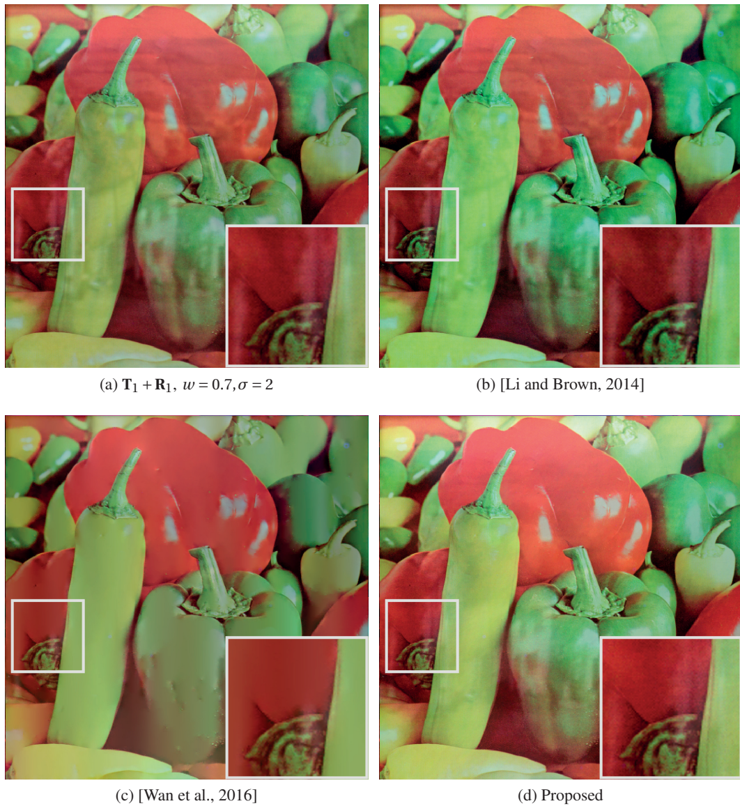
Figure 4.6 – Comparison of reflection removal methods on synthetic images with blending weight w = 0.7 . Compared to [Li and Brown, 2014] and [Wan et al., 2016] our method gives superior color reproduction and reflection suppression results. Best viewed on screen.
