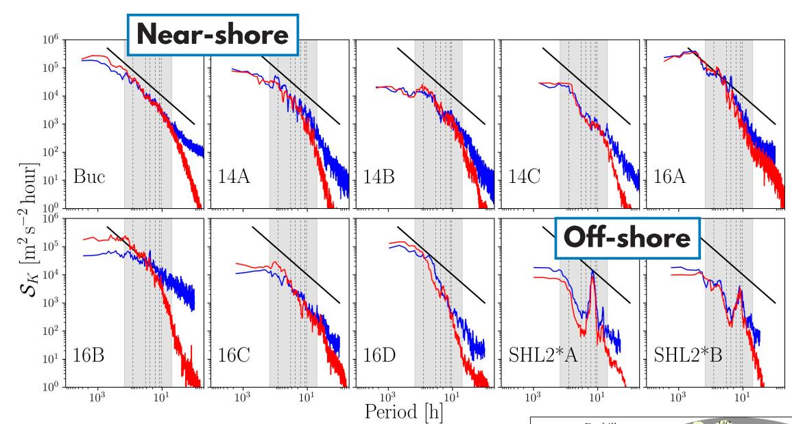
Kinetic energy spectra from observational and model data. The vertical lines mark, from left to right, the following periods in hours: 81.5 (L1), 33.3 (L3), 24 (diurnal), 16.5 (inertial/Coriolis), 12 (semidiurnal) and 10.6 (T1). The thick black line is a guide for the eye (power law with exponent -1). The gray shaded area approximately identifies the internal wave range.
