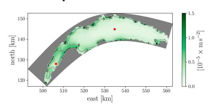
Green shading: advective component of acceleration. Contours: forcing minus dissipation (mainly bottom friction). Gray (black) contours: 10<sup>-6</sup> (10<sup>-5</sup>) m s<sup>-2</sup>. Average over the period from 2016-07-01 to 2016-09-30, using bihourly averaged diagnostics.
