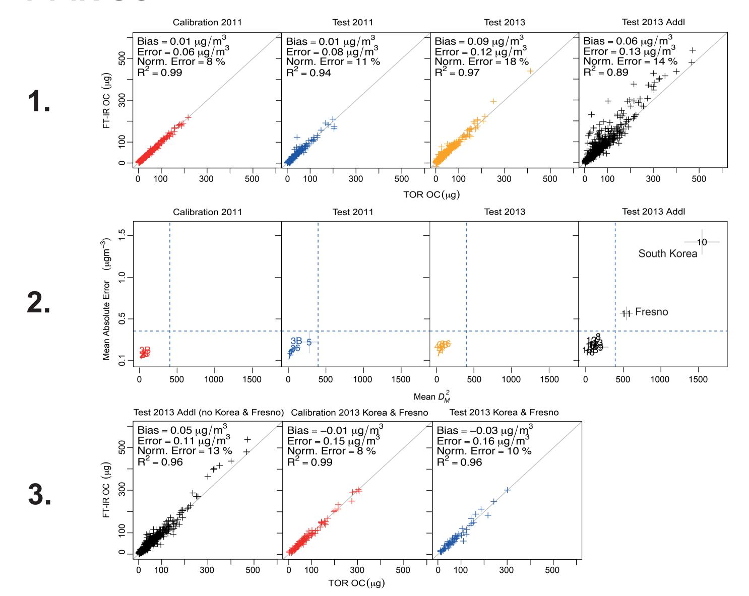
FT-IR and PLS accurately predict (0.94≤R²≤0.97) TOR OC values from PTFE ambient samples collected at the same sites and in the same or different years of the ones used for the calibration (blue and orange scatterplots).
