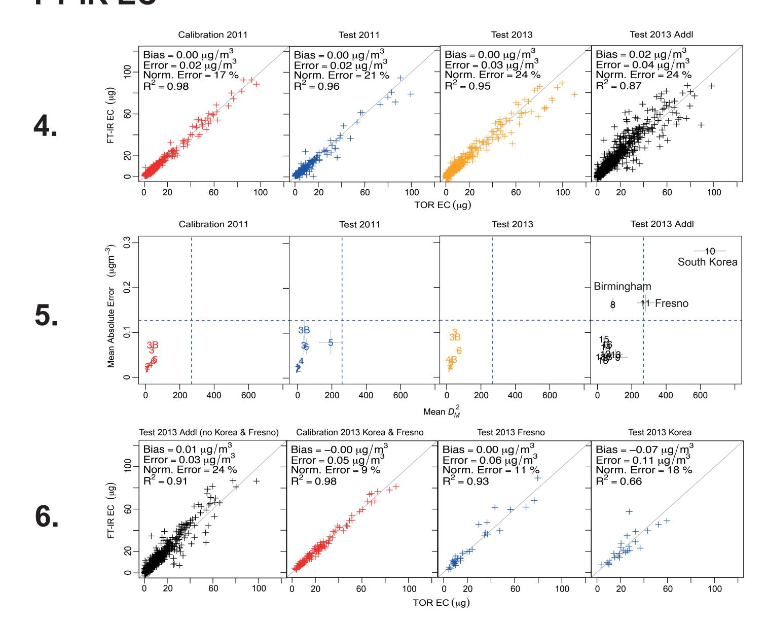
FT-IR and PLS accurately predict (0.95≤R²≤0.96) TOR EC values from PTFE ambient samples collected at the same sites and in the same or different years of the ones used for the calibration (blue and orange scatterplots).
