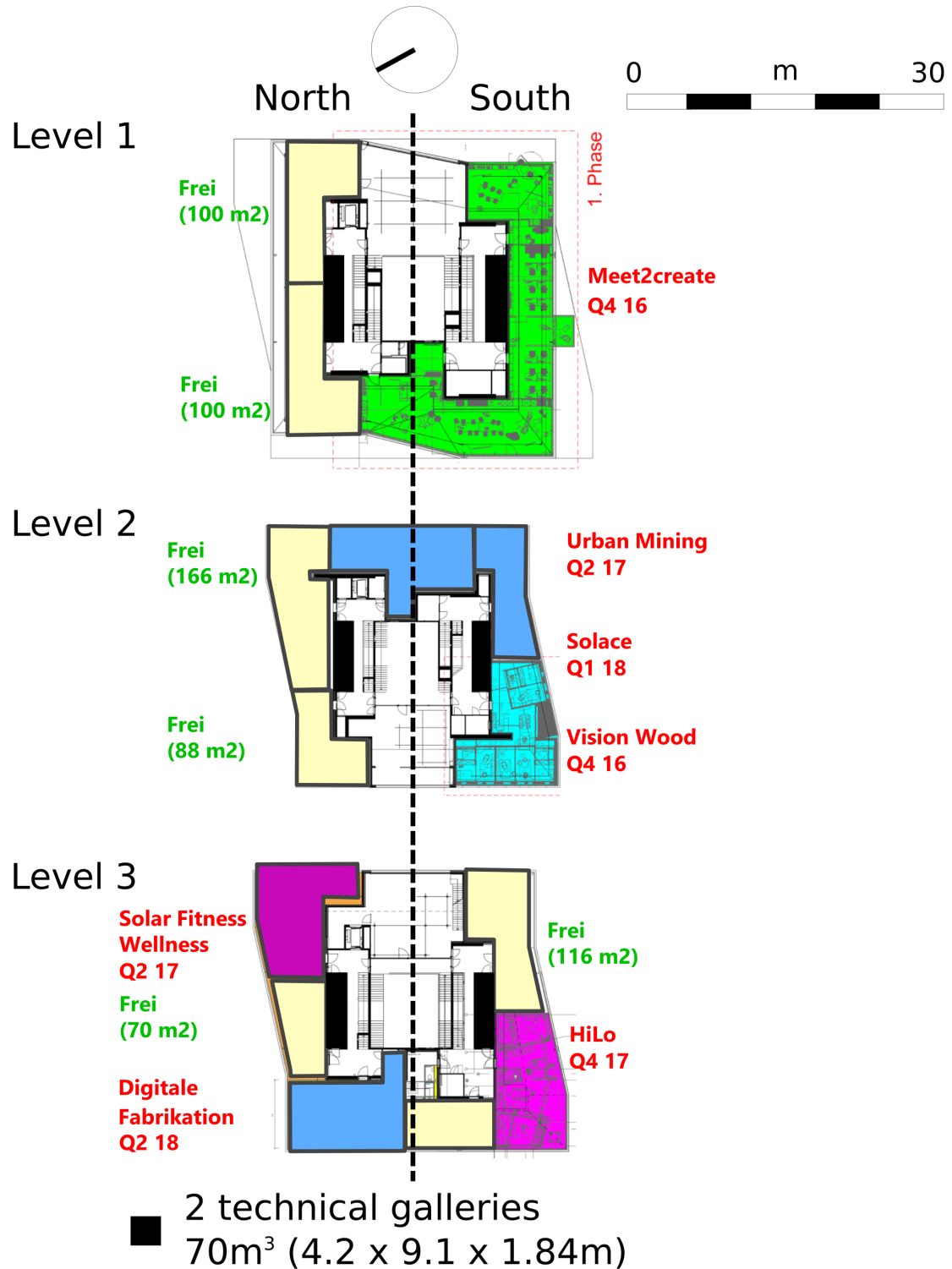
Figure 5: Planned and future units of the NEST platforms with "North" and "South" technical galleries in the middle (black) – Source: Empa.
