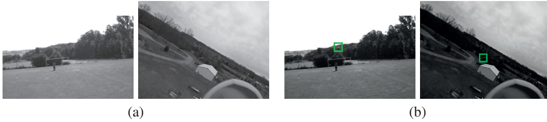
Figure 1: Detecting a small flying object against a complex moving background. (a) It is almost invisible to the human eye and hard to detect from a single image. (b) Yet, our algorithm can find it by using appearance and motion cues.
