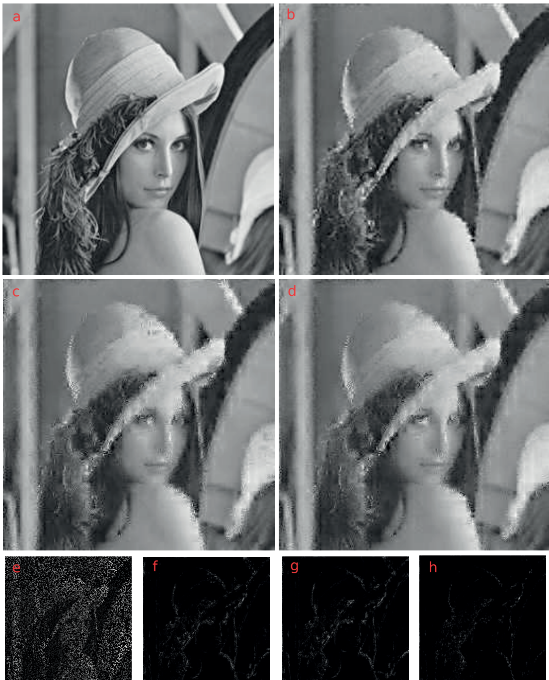
Figure 2.14 – Example results for inpainting "Lena" a: Truth. b: VB-Lap-tree . c: MAP-Lap-tree. d: VB-Lap-fact. e: y (Input: 25% of a). f: |c - a| . g: |d - a| . h: |b - a| .
