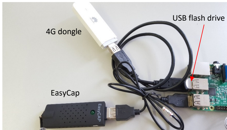
Figure 5. Connection of different USB devices: 4G dongle, USB flash drive and EasyCAP (converts composite video to USB-compatible format).
