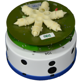
Fig. 5. A Khepera IV robot equipped with an odor sensing board and an anemometer board stacked on top.
