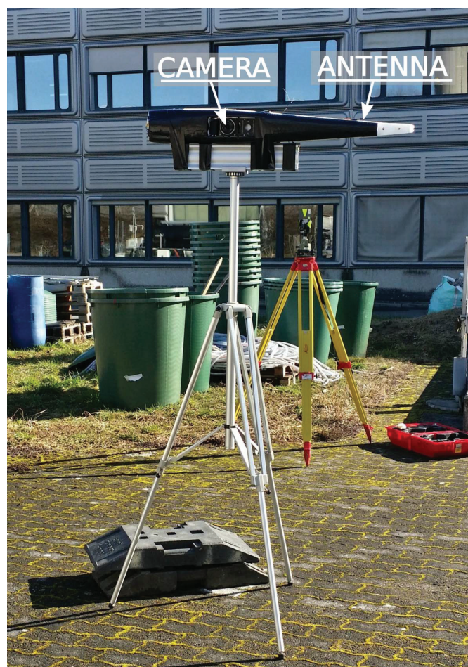
Figure C.1 – The lever-arm calibration setup. The fuselage without wings and with the camera and antenna pointing towards the calibration field.
