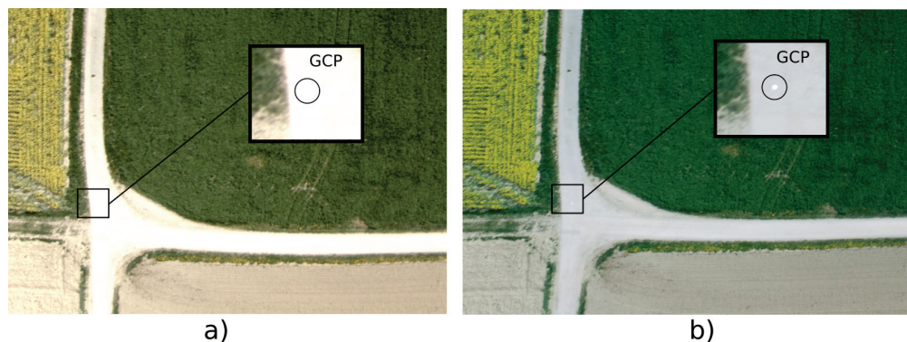
Figure 7.2 – Automatic and manual image conversion from raw to JPEG format; a) automatic conversion using the senseFly eMotion2, b) manual correction using a photo editor. The image was taken with the Canon PowerShot S110 camera having 12.1 Mpix resolution (Canon Inc. [2016]).
