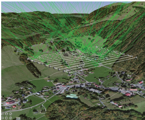
Figure 3.12 – Visibility of GNSS satellites for certain points represented by imaginary rays between sampled trajectory and satellites.
