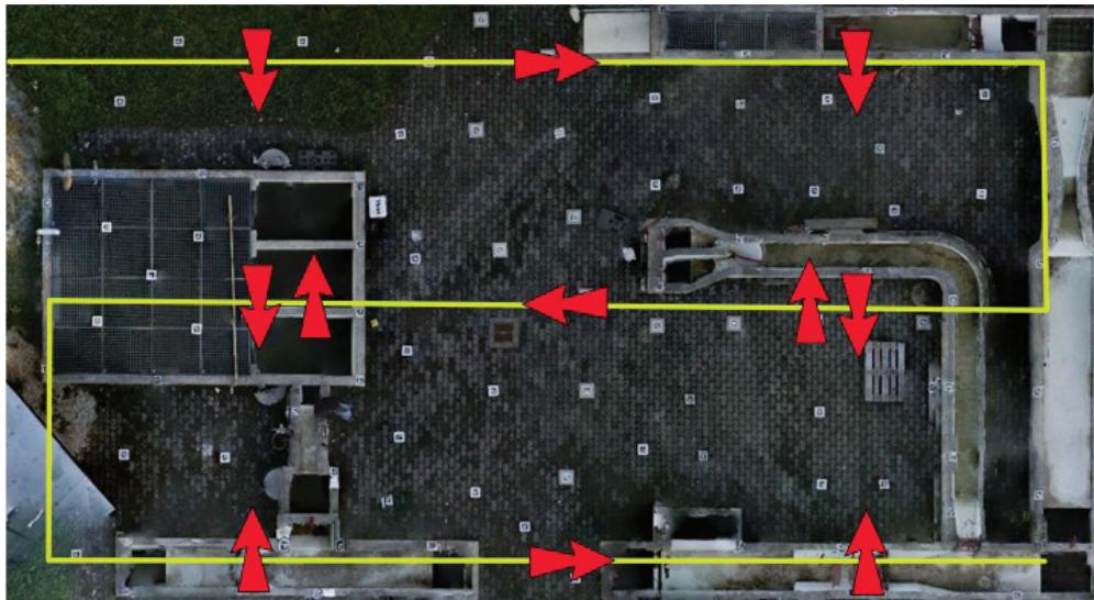
Figure 6.15 – Camera calibration flight over a dedicated field. The yellow line symbolises the flown trajectory, the red arrows symbolise the camera orientation during the image acquisition.
