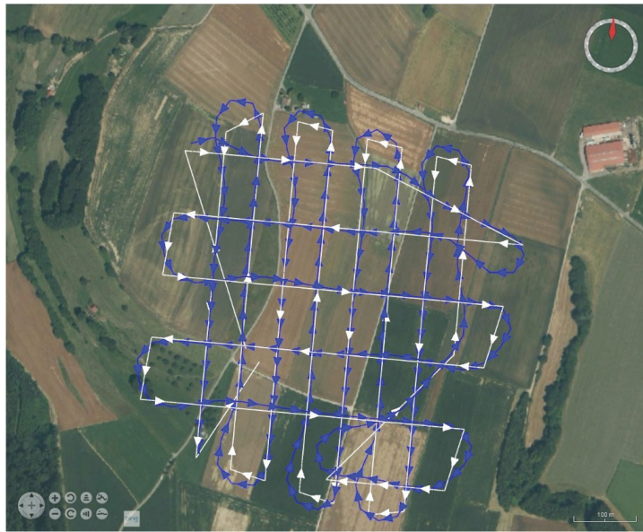
Figure 3.14 – Post-mission analysis; blue path: the executed flight, white path: the planned path.
