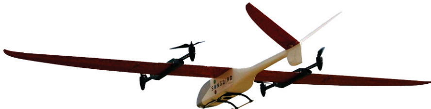
Figure 2.6 – Fixed-wing UAV with VTOL capabilities Songbird (Aerolution GmbH [2016]). Depending on the payload, this UAV fits into MAV or Mini UAV categories.
