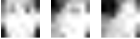
Figure 3. Examples of trained colour patterns corresponding to pan ( \varphi ) angle values of 0, 45 and 90 degrees and tilt ( \psi ) angle value 0.
