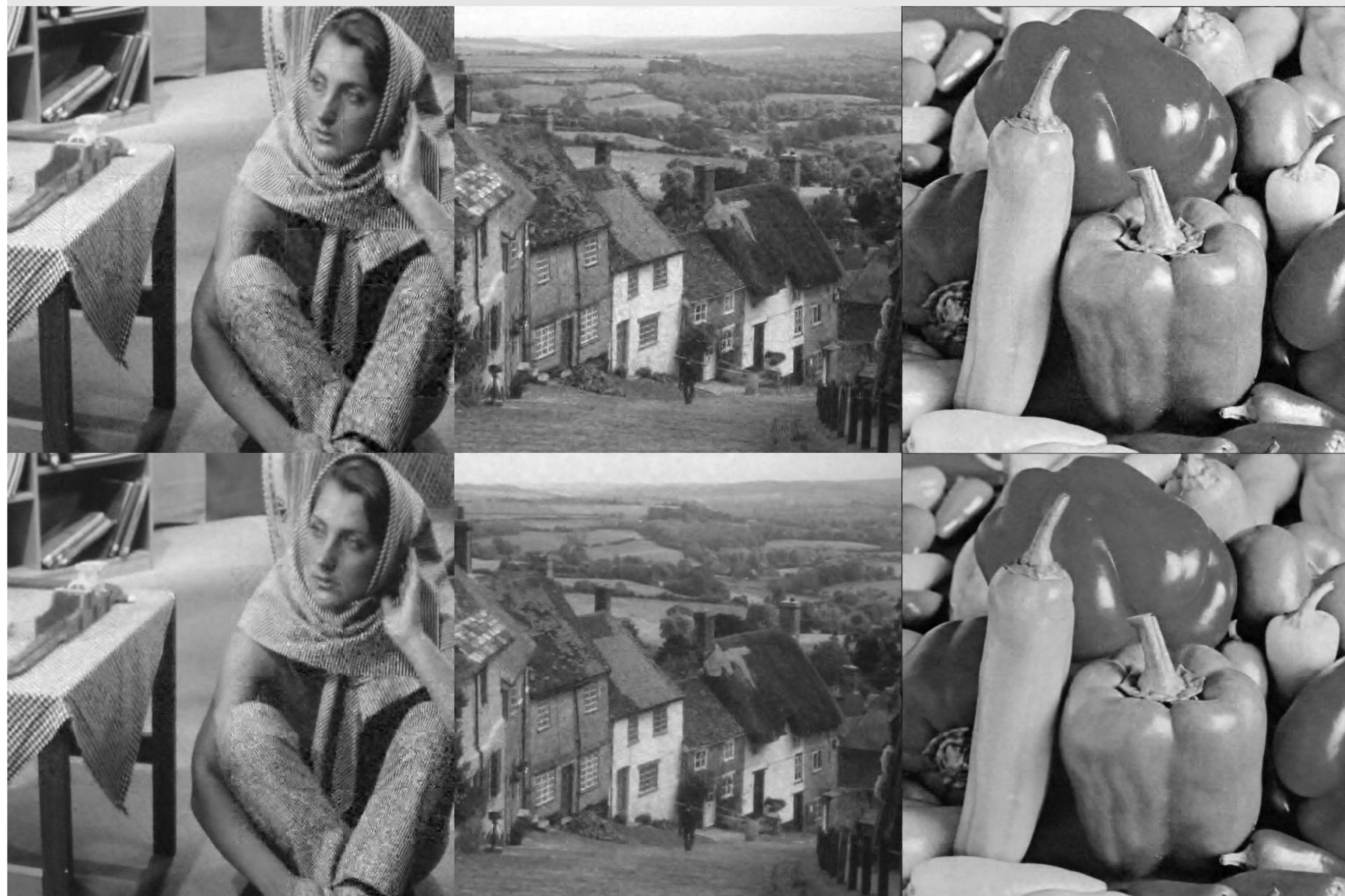
Figure Test images reconstructed for a measurement rate M_B/N_B^2 = 0.3 (first row) with tiled SARA and (second row) with LEFISTA (50 layers)
