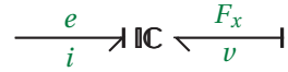
Figure 4.4 – Bond graph representation of the electromagnet transducers imposing preferred integrative causalities on its ports.
