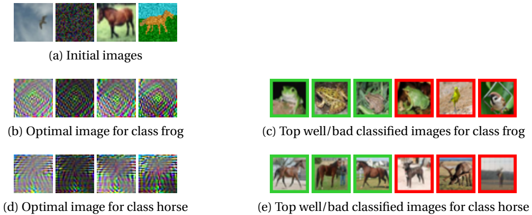
Figure B.1 – Images in B.1a are the initial images used for gradient descent. The images below are the ones to which the algorithms have converged after 300 iterations of gradient descent, when the target class was frog (images B.1b) and horse (images B.1d). Pictures B.1c and B.1e are the images of the test set of CIFAR with a high response in the two considered classes. A green frame indicates that the image is correctly classified as a frog/horse, and the red frame indicated that the image is misclassified. We note that even though the bird of picture B.1c has a positive score in the class bird, it has a bigger score in class frog, possibly due to the perch.
