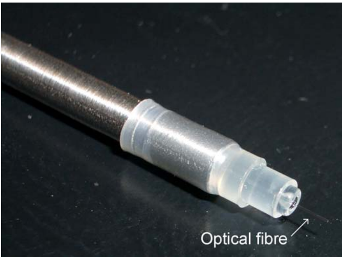
Fig. 2 – Optical tool for local neuronal stimulation.
