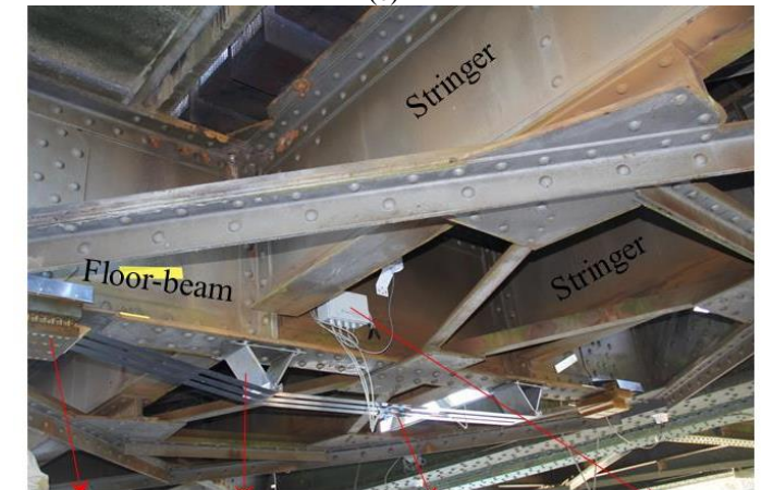
Friction clamp Column Strain gauges bonded to CFRP laminates Wireless sensor network node
